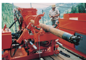
Pipe Roof, Water Service Water Remove, Anchoring It achieves excellent results for drilling of long holes and hard formations using the Down The Hole Hammer. Top-Hammer applications are available.
